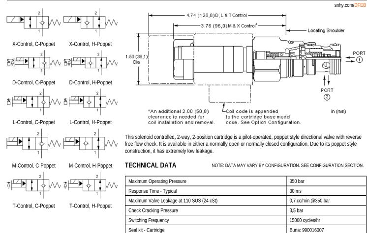
• Please verify cartridge clearance requirements when choosing a Sun manifold. Different valve controls and coils require different clearances.
