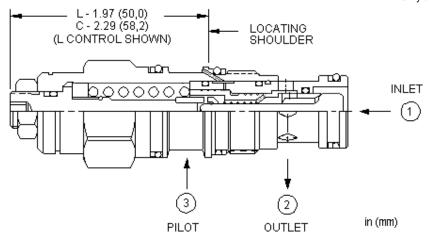
Counterbalance valves with pilot assist are meant to control an overrunning load. The check valve allows free flow from the directional valve (port 2) to the load (port 1) while a direct-acting, pilot-assisted relief valve controls flow from port 1 to port 2. Pilot assist at port 3 lowers the effective setting of the relief valve at a rate determined by the pilot ratio.
