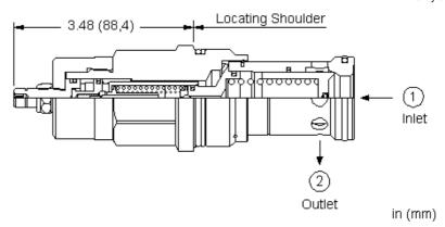
Pilot-operated, anti shock relief cartridges limit maximum system pressure and also limit the rate of pressure rise. The valve opens and then ramps closed at a constant speed, independent of settings and flows. The adjust screw determines the maximum (relief) setting and the minimum (threshold) setting.
