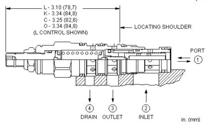
Direct-acting, pressure reducing/relieving valves reduce a high primary pressure at the inlet (port 2) to a constant reduced pressure at port 1, with a full-flow relief function from port 1 to tank (port 3). Draining port 4 makes the valve insensitive to pressure at port 3. These valves incorporate a damped construction for stable operation allowing the use of high reduced pressure.
