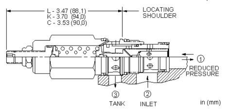
Direct-acting, pressure reducing/relieving valves reduce a high primary pressure at the inlet (port 2) to a constant reduced pressure at port 1, with a full-flow relief function from port 1 to tank (port 3). These valves incorporate a damped construction for stable operation allowing the use of high reduced pressure.
