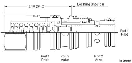
This valve is a 2-way, 2-position proportional throttle. Ports 2 and 3 are normally closed. Pilot pressure at port 1 creates a metering orifice between port 2 and 3 that is proportional to the pressure at 1. The force balance of the flow forces, spring and pilot pressure results in a degree of partial self-compensation as the load pressure changes.
