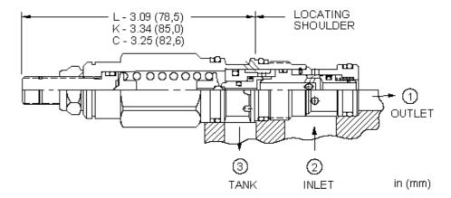
The relief-before-check cartridge is a CavitySaver™ (multi-function) valve incorporating a direct-acting relief tee'd in before a check function. When the pressure at the inlet (port 2) reaches the relief valve setting, the valve starts to open to tank (port 3), throttling flow to limit the pressure rise. The check valve flow is from the inlet (port 2) to the system port (port1). These valves are smooth and quiet, essentially zero leak, dirt tolerant, immune to silting and are very fast.
