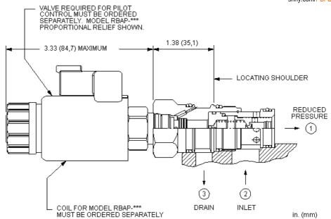
This valve is a normally open modulating element that incorporates an integral pilot control cavity. The pilot control cavity will accept any T-8A pressure control cartridge. The valve reduces a high primary pressure at the inlet (port 2) to a constant reduced pressure at port 1. The pilot cartridge's setting determines the difference in pressure between reduced pressure (port 1) and the drain (port 3).
