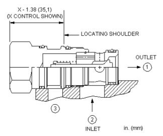
Free-flow, side-to-nose cheater check valves function as a standard 2-port check valve in a 3-port cavity with port 3 of the cartridge blocked off. These valves are useful in circuits where a check valve is required in an existing three port cavity.
