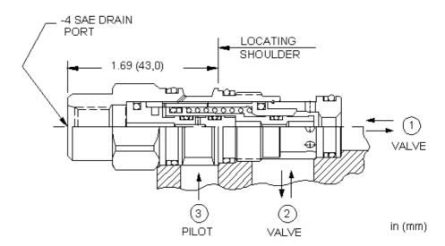
This is a normally open, balanced poppet, switching element. When the external vent port is blocked, the poppet remains in the open position. Venting the external port shifts it to the closed position, provided there is sufficient pressure at port 3.
