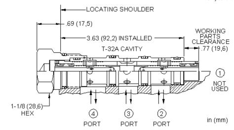
Synchronizing flow divider/combiners are sliding-spool, pressure-compensated devices used to split flow in one direction and combine flow in the opposite direction. With a sychronizing feature, these valves can be used to allow two hydraulic cylinders to fully stroke and synchronize at the end of the stroke. When the first cylinder has reached the end of its stroke, a pressure-compensated, reduced flow is metered to or from the second cylinder until it also reaches the end of its stroke.
