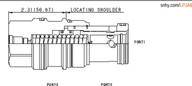
These normally open modulating elements with an internal orifice between port 1 and port 3 can be used as a main-stage reducing valve. The valve can be controlled remotely using a pilot relief or pilot solenoid valve.
