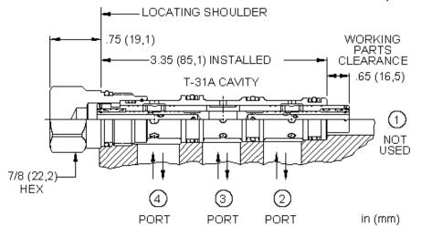
High accuracy, closed-center flow divider/combiners are sliding-spool, pressure-compensated devices used to split flow in one direction and combine flow in the opposite direction. These valves may be used to accurately control two or more cylinders or hydraulic motors where bidirectional operation is required.
