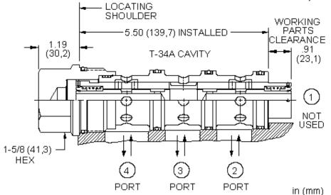
Closed-center flow divider/combiners are sliding-spool, pressure-compensated devices used to split flow in one direction and combine flow in the opposite direction. These valves may be used to accurately control two or more cylinders or hydraulic motors where bidirectional operation is required.
