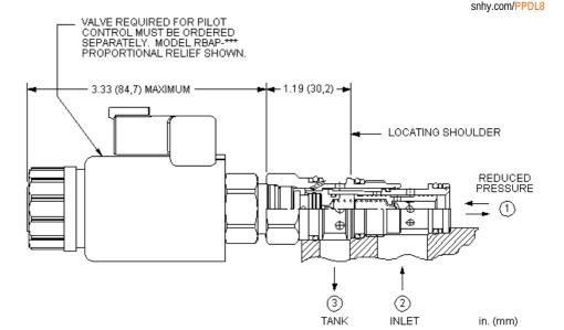
This valve is a 3-way, normally open modulating element that incorporates an integral pilot control cavity. The pilot control cavity will accept any T-8A pressure control cartridge. The valve reduces a high primary pressure at the inlet (port 2) to a constant reduced pressure at port 1, with a full flow relief function from port 1 to tank (port 3). The pilot cartridge's setting determines the difference in pressure between reduced pressure (port 1) and the tank (port 3).
