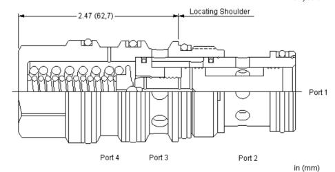
This valve is a 2-way, 2-position proportional throttle. Ports 2 and 3 are normally closed. Pilot pressure at port 1 creates a metering orifice between port 2 and 3 that is proportional to the pressure at 1. The force balance of the flow forces, spring and pilot pressure results in a degree of partial self-compensation as the load pressure changes.
