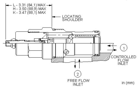
Needle valves with reverse-flow check are fully adjustable orifices used to regulate flow. They are infinitely adjustable from fully closed up to the maximum orifice diameter. An integral high-capacity check valve provides unrestricted flow from port 2 to port 1. They are not pressure compensated.
