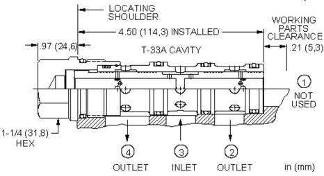
Flow dividers are sliding-spool, pressure-compensated devices used to split oil flow to two different branches of a circuit in a designated ratio. These valves are suitable for applications that use the following: unidirectional hydraulic motors, hydraulic cylinders where flow division in one direction only is required, and multiple circuits that are serviced from one pump supply.
