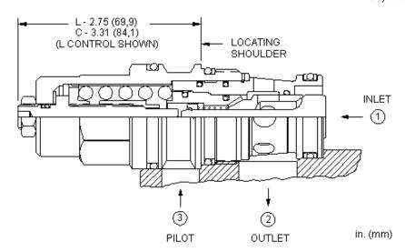
Counterbalance valves with pilot assist are meant to control an overrunning load. The check valve allows free flow from the directional valve (port 2) to the load (port 1) while a direct-acting, pilot-assisted relief valve controls flow from port 1 to port 2. Pilot assist at port 3 lowers the effective setting of the relief valve at a rate determined by the pilot ratio.
