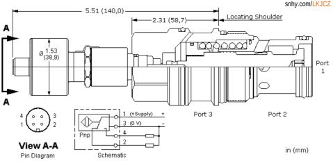
These unbalanced poppet, logic valves are 2-way switching elements that are spring-biased closed. Pressure at either work port 1 or 2 will further bias the valve to the closed position while pressure at port 3 will tend to open it. The force generated at port 3 must be greater than the sum of the forces acting at port 1 and port 2 plus the spring force for the valve to open. NOTE: The pilot area (port 3) is 1.8 times the area at port 1 and 2.25 times the area at port 2.
