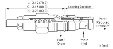
Direct-acting, pressure reducing valves reduce a high primary pressure at the inlet (port 2) to a constant reduced pressure at port 1. These valves incorporate a damped construction for stable operation allowing the use of high reduced pressure. This valve is open in the transition from reducing to relieving. It provides good pressure control and dynamic response.
