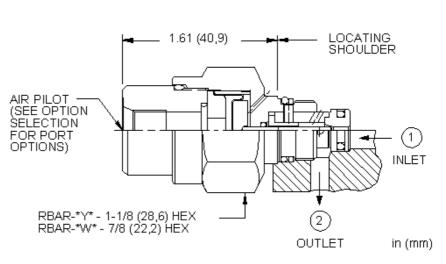
Two-port, pilot-stage, air-controlled, direct-acting relief cartridges are normally closed pressure regulating valves. When the pressure at port 1 (inlet) is sufficient to overcome the force due to the air signal, a flow path is opened from port 1 to port 2 (tank). These cartridges are designed for pilot flow applications and utilize Sun's T-8A cavity so they can be used in conjunction with Sun's pilot-operated, main-stage valves.
