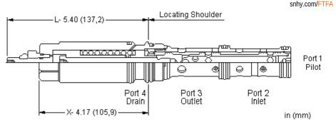
This valve is a 2-way, 2-position proportional throttle. Ports 2 and 3 are normally closed. Pilot pressure at port 1 opposes the spring and creates a variable metering orifice between port 2 and 3 that is proportional to the pressure at 1. The force balance of the flow forces, spring and pilot pressure results in a degree of partial self-compensation as the load pressure changes.
