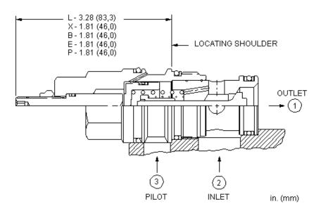
This valve is a pilot to open check valve. It has a sealed pilot, a steel seat, and is non-vented. It allows free flow from the valve (port 2) to the load (port 1) and blocks flow in the opposite direction. Pressure at the pilot (port 3) will open the valve from port 1 to port 2. Pilot pressure needed at port 3 to open the valve is directly proportional to the load pressure at port 1. Pressure at port 2 directly opposes pilot pressure.
