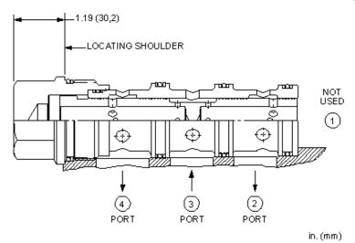
Flow dividers are sliding-spool, pressure-compensated devices used to split oil flow to two different branches of a circuit in a designated ratio. These valves are suitable for applications that use the following: unidirectional hydraulic motors, hydraulic cylinders where flow division in one direction only is required, and multiple circuits that are serviced from one pump supply.
