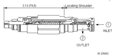
Pilot-operated, anti shock relief cartridges limit maximum system pressure and also limit the rate of pressure rise. The valve opens and then ramps closed at a constant speed, independent of settings and flows. The adjust screw determines the maximum (relief) setting and the minimum (threshold) setting.
