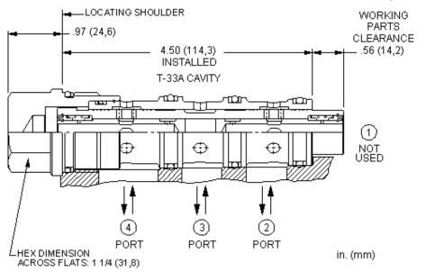
High accuracy, closed-center flow divider/combiners are sliding-spool, pressure-compensated devices used to split flow in one direction and combine flow in the opposite direction. These valves may be used to accurately control two or more cylinders or hydraulic motors where bidirectional operation is required.
