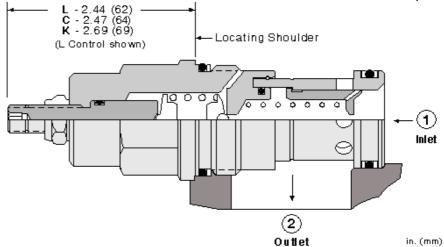
Kick-down relief cartridges act similar to a circuit breaker in an electrical system. The valves will kick completely open and remain open once the pressure at the inlet (port 1) exceeds the valve setting, creating an unrestricted flow path from port 1 to tank (port 2). The valve remains open as long as the pressure at port 1 exceeds the pressure at port 2. To reset the valve, flow from port 1 to port 2 must cease and pressure at port 2 must be equal to or greater than the pressure at port 1.
