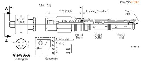
This valve is a 2-way, 2-position proportional throttle. Ports 2 and 3 are normally closed. Pilot pressure at port 1 creates a metering orifice between port 2 and 3 that is proportional to the pressure at 1. The metering passage is self-compensating.
