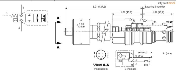
These unbalanced, pilot-to-close logic valves are 2-way switching elements that are spring biased closed. Pressure at either work port 1 or 2 will oppose the spring and tend to open the valve while pressure at port 3 will tend to close it. The force generated by the pressure at port 3, plus the spring force, must be greater than the sum of the forces generated by the pressures at ports 1 and 2 for the valve to remain closed.
