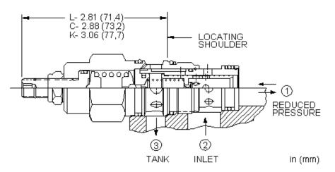
Pilot-operated, pressure reducing/relieving valves reduce a high primary pressure at the inlet (port 2) to a constant reduced pressure at port 1, with a full-flow relief function from port 1 to tank (port 3).
