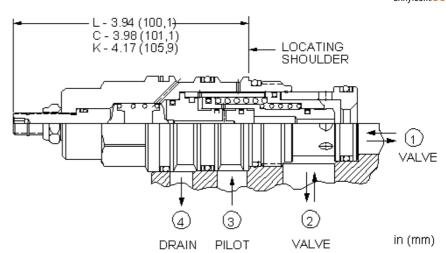
This is a normally open, balanced poppet, switching element. When pilot pressure is applied to port 3, the poppet remains open until the pilot pressure reaches the setting established by the integral pilot relief stage, at which point the poppet shifts to the closed position.
