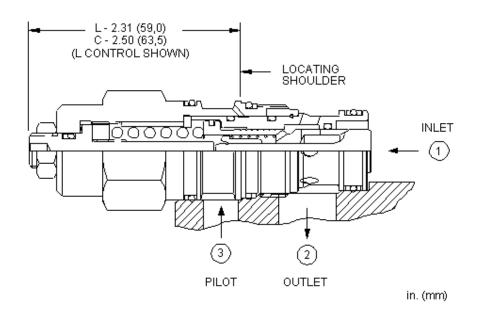
Counterbalance valves with pilot assist are meant to control an overrunning load. The check valve allows free flow from the directional valve (port 2) to the load (port 1) while a direct-acting, pilot-assisted relief valve controls flow from port 1 to port 2. Pilot assist at port 3 lowers the effective setting of the relief valve at a rate determined by the pilot ratio.
