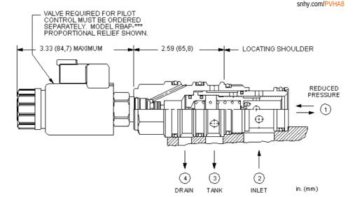
This valve is a 3-way, normally open modulating element, externally drained, that incorporates an integral pilot control cavity. The pilot control cavity will accept any T-8A pressure control cartridge. The valve reduces a high primary pressure at the inlet (port 2) to a constant reduced pressure at port 1, with a full flow relief function from port 1 to tank (port 3). The pilot cartridge's setting determines the difference in pressure between reduced pressure (port 1) and the drain (port 4).
