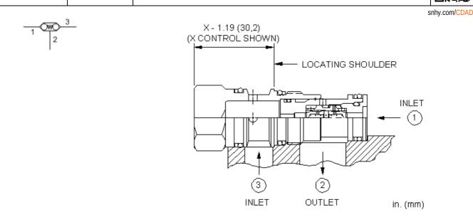
The back-to-back check valve combines two simple check valves into a single cartridge. It connects the work port with the higher pressure to the signal or common port. The signal is sensed at port 2.
