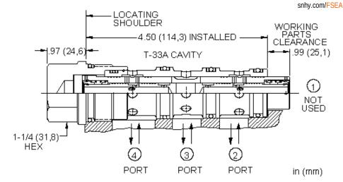
Closed-center flow divider/combiners are sliding-spool, pressure-compensated devices used to split flow in one direction and combine flow in the opposite direction. These valves may be used to accurately control two or more cylinders or hydraulic motors where bidirectional operation is required.
