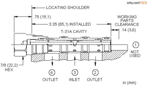
Flow dividers are sliding-spool, pressure-compensated devices used to split oil flow to two different branches of a circuit in a designated ratio. These valves are suitable for applications that use the following: unidirectional hydraulic motors, hydraulic cylinders where flow division in one direction only is required, and multiple circuits that are serviced from one pump supply.
