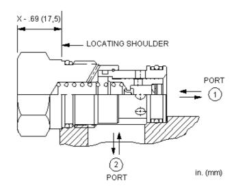
Flow fuse cartridges are used to maintain the position of a hydraulic actuator in the event of a hose or line break. The valve allows flow to and from the actuator but closes instantly if flow from the actuator exceeds the setting of the valve. NOTE: Because the valve responds so rapidly, it is sensitive to any transient flow above the valve setting.
