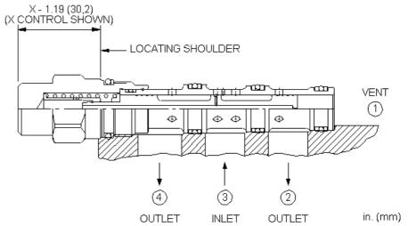
This is a vent-to-shift, 2-position, diverter valve that is normally closed. When port 1 is vented, the pressure differential between port 3 and port 1 exceeds the spring force causing the valve to shift, thereby connecting port 3 with ports 2 and 4.
