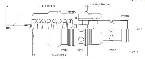
This valve is a 2-way, 2-position proportional throttle. Ports 2 and 3 are normally closed. Pilot pressure at port 1 creates a metering orifice between port 2 and 3 that is proportional to the pressure at 1. The force balance of the flow forces, spring and pilot pressure results in a degree of partial self-compensation as the load pressure changes.
