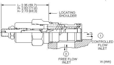
Needle valves with reverse-flow check are fully adjustable orifices used to regulate flow. They are infinitely adjustable from fully closed up to the maximum orifice diameter. An integral high-capacity check valve provides unrestricted flow from port 2 to port 1. They are not pressure compensated.
