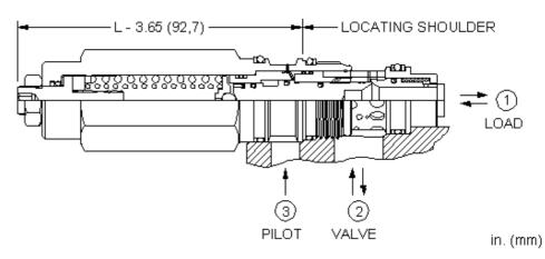
Load reactive, load control valves with pilot assist combine two valves; a check valve and a relief valve. The check valve allows free flow from the directional valve (port 2) to the load (port 1) while a direct-acting, pilot-assisted relief valve controls flow from port 1 to port 2. Pilot assist at port 3 lowers the effective setting of the relief valve at a rate determined by the pilot ratio.
