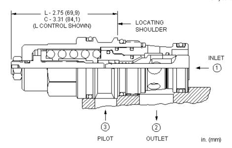
Counterbalance valves with pilot assist are meant to control an overrunning load. The check valve allows free flow from the directional valve (port 2) to the load (port 1) while a direct-acting, pilot-assisted relief valve controls flow from port 1 to port 2. Pilot assist at port 3 lowers the effective setting of the relief valve at a rate determined by the pilot ratio.
