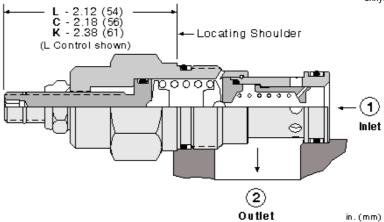
Kick-down relief cartridges act similar to a circuit breaker in an electrical system. The valves will kick completely open and remain open once the pressure at the inlet (port 1) exceeds the valve settting, creating an unrestricted flow path from port 1 to tank (port 2). The valve remains open as long as the pressure at port 1 exceeds the pressure at port 2. To reset the valve, flow from port 1 to port 2 must cease and pressure at port 2 must be equal to or greater than the pressure at port 1.
