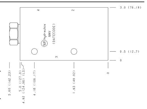
Flow dividers are sliding-spool, pressure-compensated devices used to split oil flow to two different branches of a circuit in a designated ratio. These valves are suitable for applications that use the following: unidirectional hydraulic motors, hydraulic cylinders where flow division in one direction only is required, and multiple circuits that are serviced from one pump supply.
