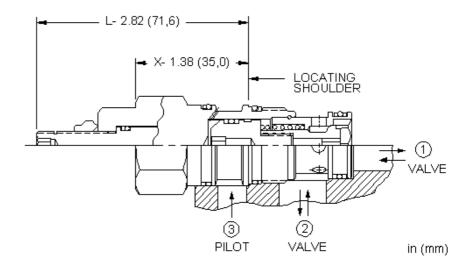
These unbalanced poppet, logic valves are 2-way switching elements that are spring-biased closed. Pressure at either work port 1 or 2 will further bias the valve to the closed position while pressure at port 3 will tend to open it. The force generated at port 3 must be greater than the sum of the forces acting at port 1 and port 2 plus the spring force for the valve to open. NOTE: The pilot area (port 3) is 1.8 times the area at port 1 and 2.25 times the area at port 2.
