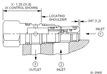
The single ball shuttle connects the higher of two work ports to the signal or common port. The signal is sensed at port 3.
