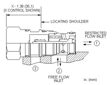
Free-flow, side-to-nose cheater check valves with a bypass orifice function as a 2-port check valve in a 3-port cavity. They allow free flow from port 2 to port 1 with a customer specified orifice that controls flow from port 1 to port 2. Port 3 of the cartridge is blocked off.
