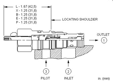
This valve is a pilot to open check valve. It has a sealed pilot, a steel seat, and is non-vented. It allows free flow from the valve (port 2) to the load (port 1) and blocks flow in the opposite direction. Pressure at the pilot (port 3) will open the valve from port 1 to port 2. Pilot pressure needed at port 3 to open the valve is directly proportional to the load pressure at port 1. Pressure at port 2 directly opposes pilot pressure.
