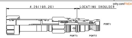
This valve is a 3-way, meter-in, electro-proportional throttle. The flow path, unenergized, has the supply blocked at port 1 and port 2 is drained to tank at port 3. Energizing the coil generates a closing force on the spool, creating a metering orifice in the 1 to 2 direction that is proportional to the coil command current. The valve self-compensates in the 1-to-2 direction and with the addition of an external compensator will provide pressure compensated flow control.
